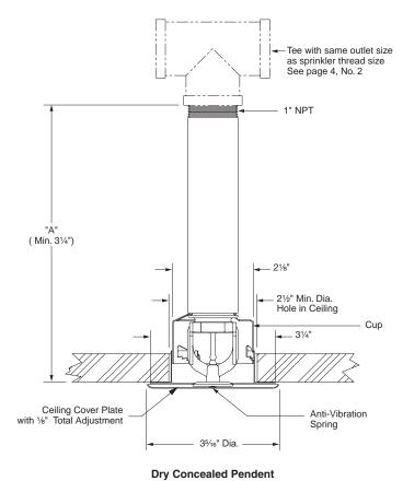
**NOTE:** The "A" dimension of a dry sprinkler which extends into freezers from wet pipe systems should be sized to provide at least 14" between the freezer's outside wall or ceiling and the wet pipe.
