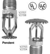
These Model V27 high pressure standard spray sprinklers are designed to produce a hemispherical spray pattern for standard commercial applications up to ordinary hazard, excluding storage applications. They have a rated working pressure of up to 250 psi (1725 kPa) and are available with either standard or quick response bulbs. The design incorporates a stateof-the-art, heat responsive, frangible glass bulb design (standard or quick response) for prompt, precise operation.
